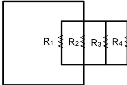
$$\begin{aligned} R_1 &= 8 \text{ } [\Omega] \\ R_2 &= 4 \text{ } [\Omega] \\ R_4 &= 2 \text{ } [\Omega] \end{aligned}$$
